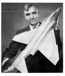
READY FOR SHIPMENT to the wind tunnel, R. T. McVeety (9323), who was design engineer for this project, holds the finished 1/20th scale model of the F-4 Phantom jet.
